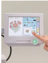
Touch Panel 999 patterns memory 40,000,000 stitches memory 触控面板999模式内存 40000000针内存
